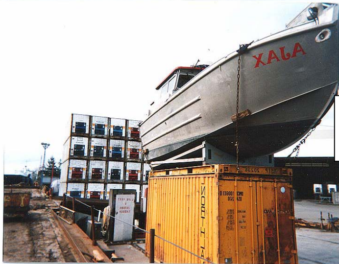
Boat and cradle are secure on platform. Note cradle does not exceed dimensions of the platform.
