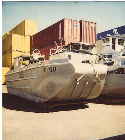
Example of a flat bottom boat. This boat does not require a cradle.
