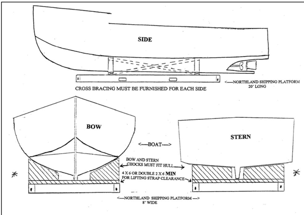
\* CHOCKS MUST BE 8' WIDE OR LESS. All bearing points must be on 8' wide shipping platforms.
