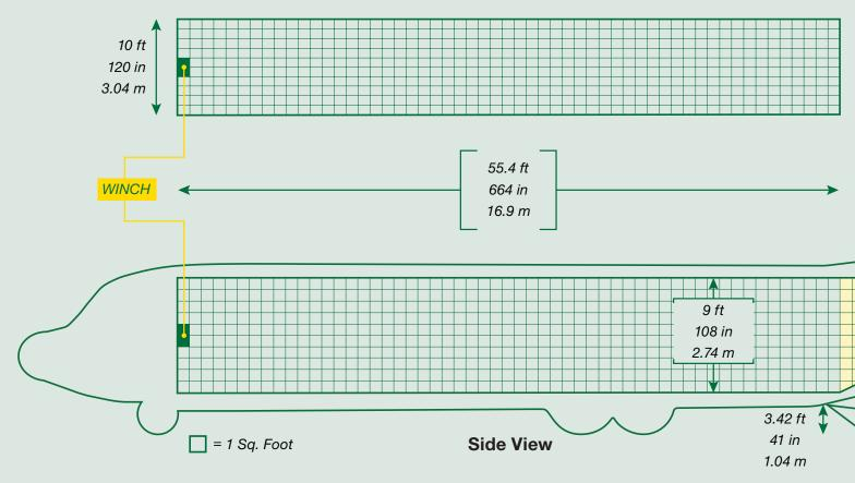
\*IMPORTANT: The drawing is only a representation of cargo space available in the L-382 Hercules. Always contact Lynden Air Cargo before producing items that you plan to fly on the aircraft.
